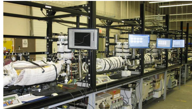
A core flooding laboratory setup for EOR / fluid transport experiments in cores under reservoir-like conditions.
