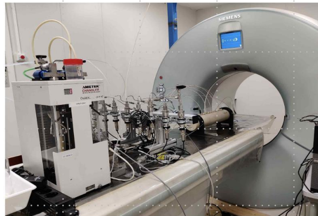
Photo of real core flooding rig setup inside a CT scanner
